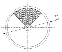
A ribbon coil could be a flame quenching device that is mounted into a flame arrester. Diameter sizing, the choice of material, the determination of capillary height and the number of ribbon coil elements depend on what they are used for.
