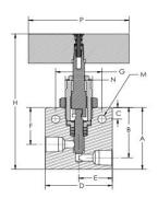
Assembly Valve 15,000 PSI, 3,8" NPT, 2-Way Straight, 2 Piece V-Stem Standard Handle
